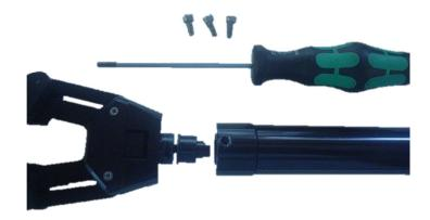
2. Remove the drive nut and spacer. Thoroughly clean the threads, drive nut, & spacer. Also, clean the inside of the housing. There are no O-rings or sealing surfaces to worry about.
